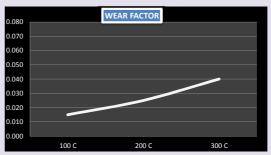
The graph displays the potential change in brake efficiency due to temperature increase. The temperature vs friction is tested as per IS 2742-1994( as per SAE J 661a) and Wear factor as per the simulation test on LINK CHASE machine. The test provides measurable frictional out put with no mechanical influence
